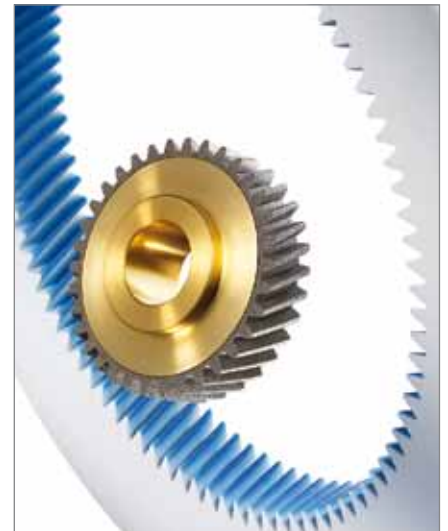
MIRA diamond dressing wheel manufactured using double-reverse plating
