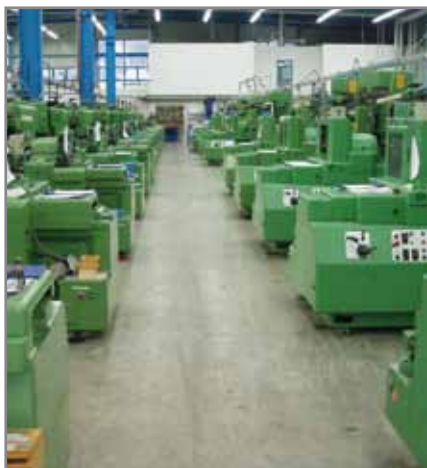
High-precision grinding of MIRA diamond dressing wheels on Maag gear grinding machines
