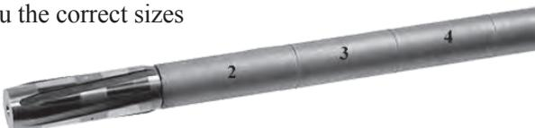
Another means of producing rifling in barrels is by Hammer Forging Rifling Mandrels. We manufacture these very precision tools in high impact carbide. The carbide mandrel has the entire depth rifling pattern ground into its surface to reflect the exact interior of the barrel.
