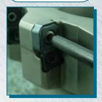
\*Tighten the insert screw completely (35in. lbs.)
