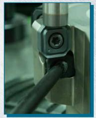
RUNOUT adjustment is completed.
