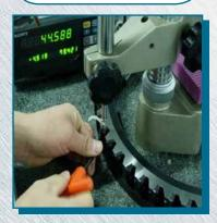
\*Do not damage the insert edge on gauge setting.
