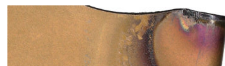
Conventional B Flank wear = .007"
