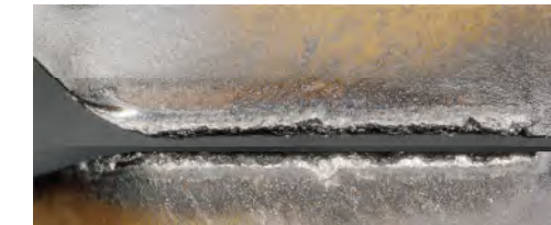
Chipping occurred due to peeling of the coating
