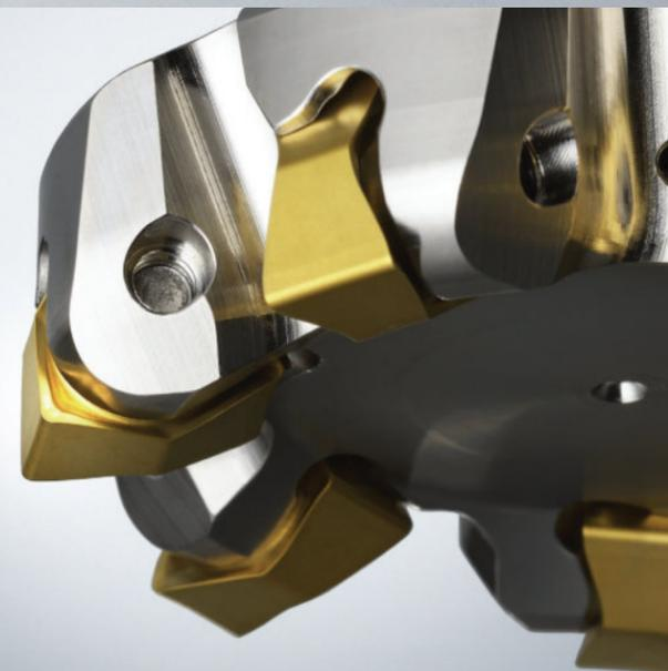
Tool body damage is negated due to the radial geometry behind the insert.
