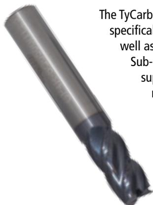
The TyCarb GP Series of 4 flute end mills have been specifically designed for today's difficult materials as well as the modern machinery now available. From Sub-Micron Carbide Rod to differential fluting and superior PVD coating the GP Series excels in difficult materials and applications.
