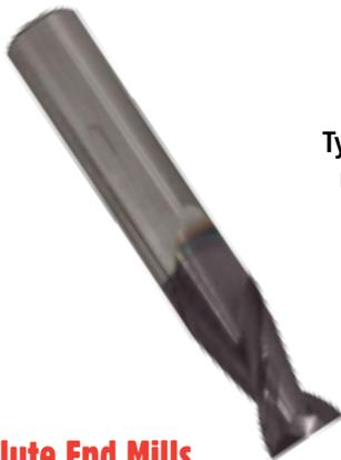
TyCarb GP Series 2 flute end mills are designed for general milling applications in low to medium carbon steels, cast iron, easy to machine stainless steels as well as aluminum, brass, bronze and copper alloys. Manufactured with square corners they are available with either cylindrical or Weldon shanks.
