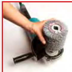
STEP 2. put flap wheel over the sleeve
