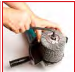
STEP 4. tighten nut with Allen wrench
