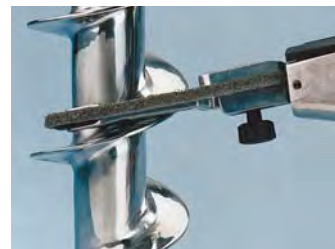
Clean and finish using non-woven nylon belts.
