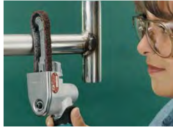
Clean and finish using non-woven nylon belts.
