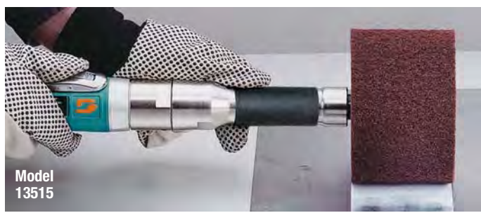
13515 Dynastraight® sets grain pattern in stainless steel.
