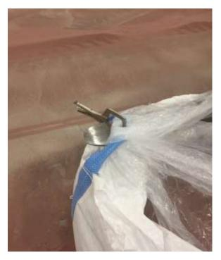
6) Lift bag and open distribution chute (sometimes the drawstring must be cut) pull down distribution chute:
