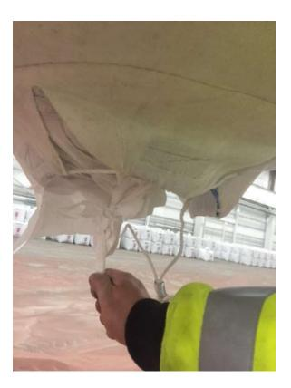
7) Slice inner liner cleanly (note; single slice pours reasonably slowly, and a 2<sup>nd</sup> slice can be made perpendicular to increase flow)
