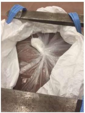
3) Cut inner line zip tie and pull upwards towards each lifting loop; pull inner liner under lifting loop:
