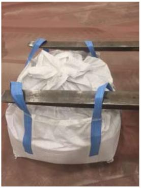
2) Open top of bulk bag duffle to expose top of inner liner:
