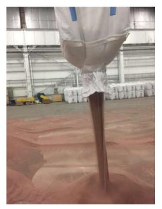
8) Garnet should flow smoothly and inner liner should not slide into distribution chute:
