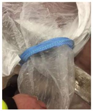
4) Wrap inner liner back over lifting loop tightly then clamp to forklift tine:
