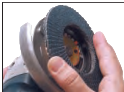
Match the CMT "loading" to the backing plate.
