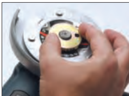
Use your standard locking nut to fasten the backing plate in place.
