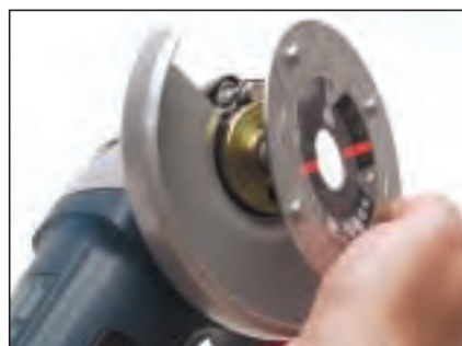
Place the backing plate on your angle grinder.
