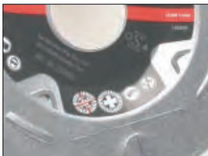
The steel CMT backing plate.
