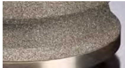
CLOSE-UP OF REVERSE-PLATED DIAMOND FORM ROLL
