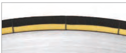
Vitrified CBN grinding tool with neutral zone.
