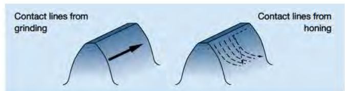
Schematic diagram of the contact lines in grinding and honing
