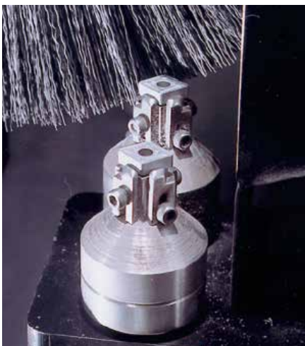
High throughput requirements make carbide inserts a good candidate for deburring with custom equipment.
