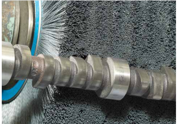
The conformability of Nylox wheels makes them excellent tools for deburring and finishing highly contoured parts like forged camshafts.
