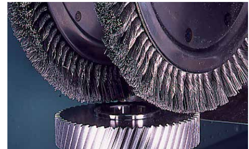
Wire wheel brushes are extremely effective for removing Class Three and Four burrs on gears and similar parts.
