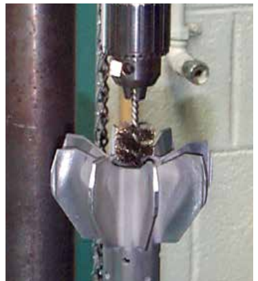
Crosshole deburring of a small casting.
