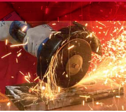
Portable snagging wheels are ideal for targeted heavy stock removal applications.
