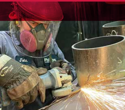
Weld blending on a stainless pressure tank with a Tiger Ceramic grinding wheel.
