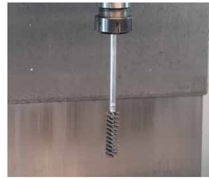
Collet ready CrossFlex brush in a CNC machine.
