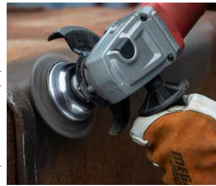
Crimped wire cup brush removing rust from a steel rail part.
