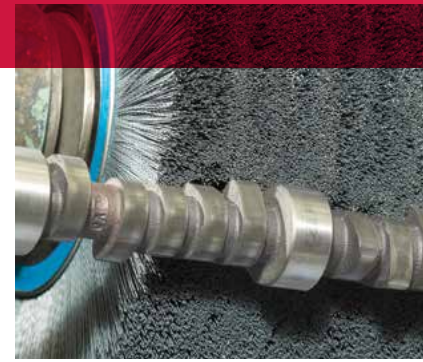
Deburring a camshaft with a Nylox wheel.
