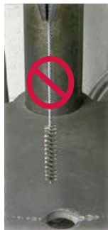
Incorrect Mounting in Chuck
