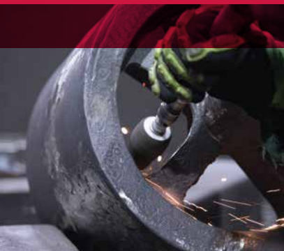
Using a cone to clean surface imperfections.
