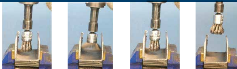
1. Insert Brush 2. Apply Power 3. Shut-Off Power 4. Remove Brush
