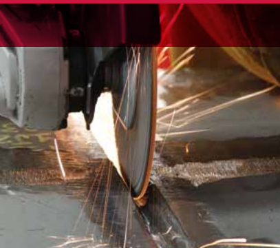
Back gouging a steel plate with a Tiger combo wheel.
