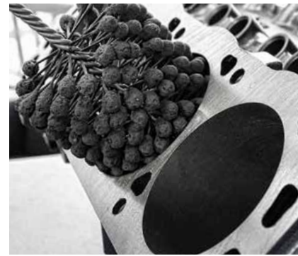
Engine cylinder head honing.
