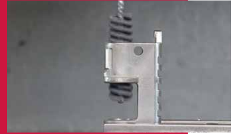
Deburring cross holes in a firearms component.
