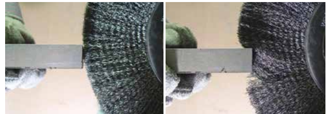
Correct Wire Tips Doing the Work
