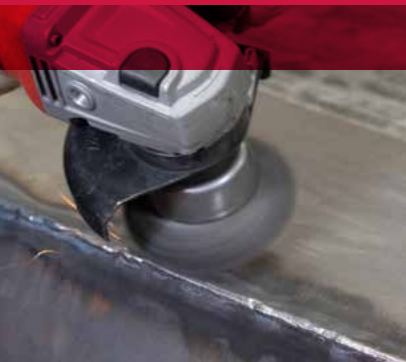
Knot wire cup brush removing heat discoloration.
