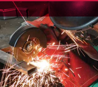
UltraCut wheel making precision cuts a steel tube stock.
