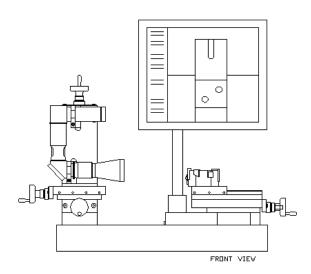
Fixture: Custom Multi-Sided Turret With Pockets, Locators, and Clamps Appropriate for a Variety of Small Workpieces Fixture Indexes Manually to Precision Pre-Set Stops
