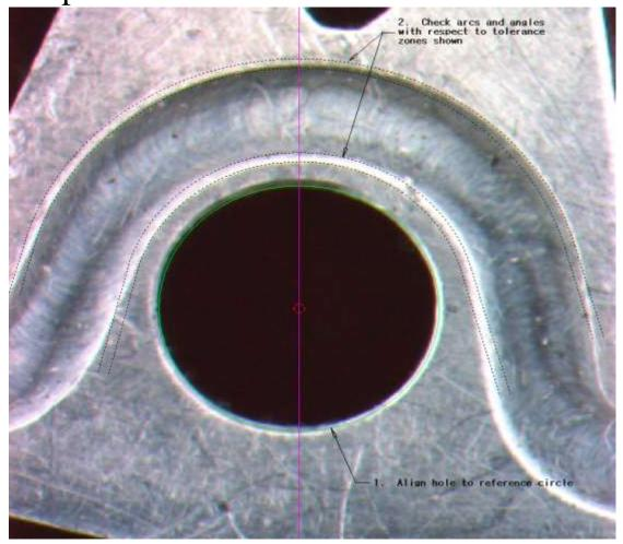
Cutting tool features are also rapidly inspected with great speed and accuracy. COVIS's zoom, up to 350X, and image enhancing allows for the most discriminating inspection of even the minutest detail. Complete with measurements, labels, time and date stamp and notes.
