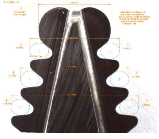
A cast aluminum housing with machined grooves.
