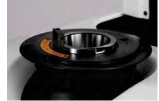
High Precision Spindle with Integrated Calibration Edge
