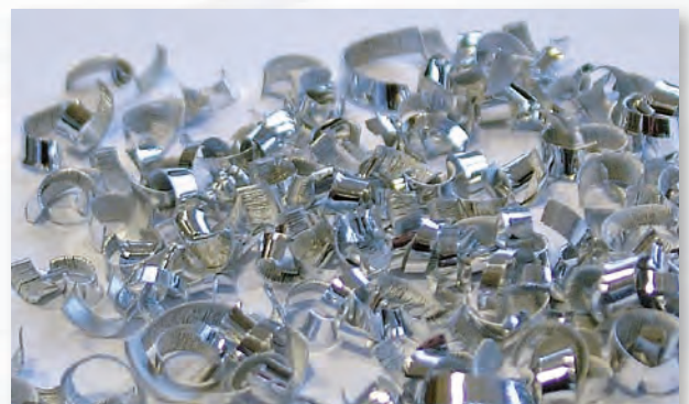
With 3D-chip breaker: Breakage chips
