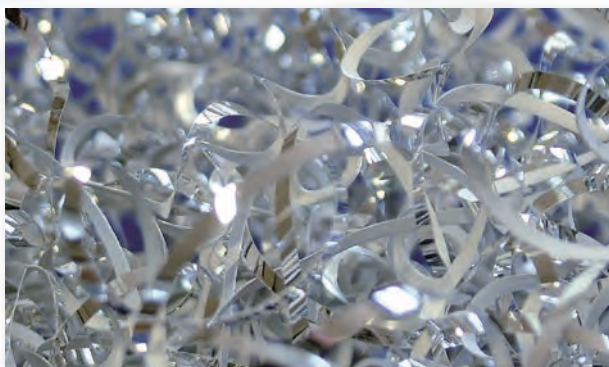
Without 3D-chip breaker: Flow chips
