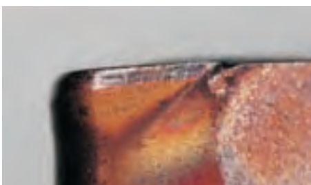
High machining temperature and simultaneous mechanical stress can lead to plastic deformation.
