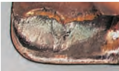
The hot chip which is being evacuated causes cratering at the rake face of the cutting edge.
