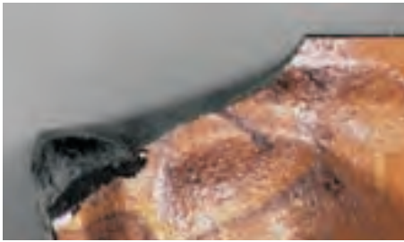
Excessive stress of the insert causes breakage.
