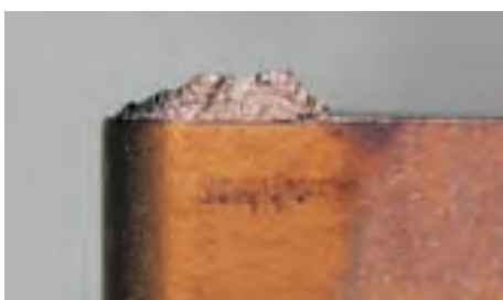
Built-up material / edges occur when the chip is not evacuated properly due to a too low cutting temperature.
