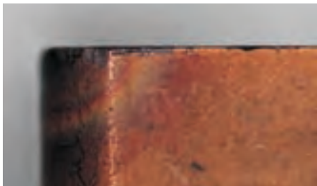
Through excessive mechanical stress at the cutting edge fracture and chipping can take place.
