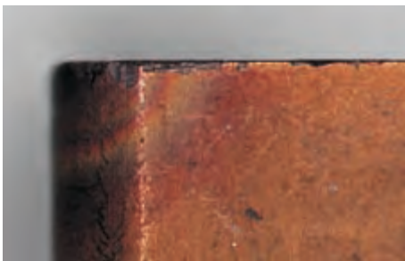
Through excessive mechanical stress at the cutting edge fracture and chipping can occur.
