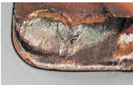
The hot chip which is being evacuated causes cratering at the rake face of the cutting edge.
