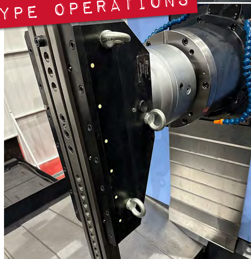
All ZX heads incorporate four Cam Lock studs that locate into the bonnet, providing exceptional rigidity.
