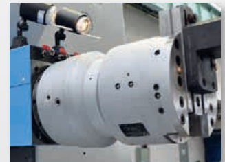
3. Engage and secure Cam Locks
