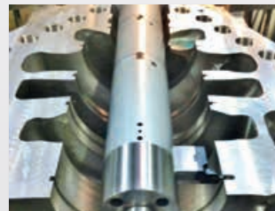
Recessing inside pump housing
