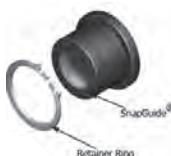
**Snap Guides** A quick-change support held in place with a snap ring. Flexible plastic SnapGuide® bushings stretch over carbide gun drill tip and contract over steel tube to stop drill whipping and vibration. Contoured hole in SnapGuide® forms perfect seal on gun drill.
