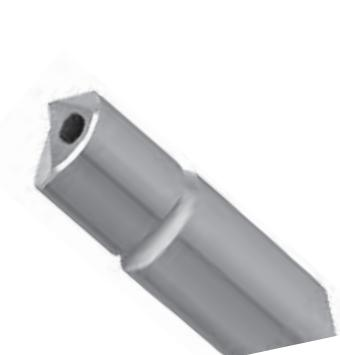
Step drills have manufacturing limitations depending on extreme diameter ranges in the steps. Special carbide developing may sometimes be necessary due to the coolant hole location. Additionally chip breakers may be required due to the lack of an inside angle which curls and breaks the chips under normal circumstances. Ideally using this type of drill yields virtually no eccentricity between diameters.
