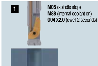
Minimum internal coolant pressure: 280 PSI (19.3 BAR)
