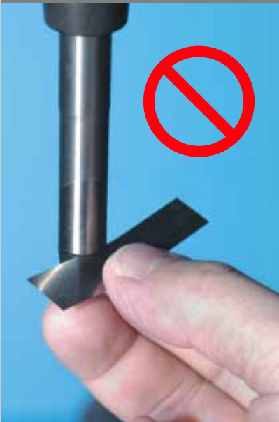
Figure 3a. Shim should NOT enter intersection
