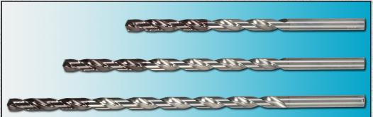
Ingersoll introduces additions to the Drill•InXL lines, for deep hole drilling up to 20xD. This drill series has optimized geometries for smooth chip evacuation with low cutting forces. A pecking cycle is not required – these drills help produce high productivity machining. These drills provide the customer with reliable machining and excellent cost savings and are designed to work with M.Q.L Systems.
