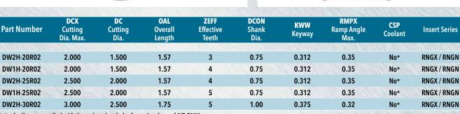
\* Cutter bodies are supplied with through coolant holes for optional use of AIR ONLY.
