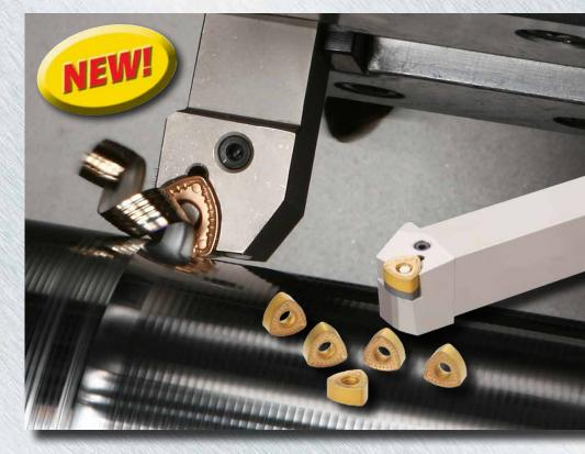
Ingersoll introduces a new, specialized turning insert for ultra high feed machining up to .118 inches per revolution (3.0mm/rev). The T-Feed insert has been developed to provide exceptionally high feed rates with a surprisingly smooth cutting action at cutting depths up to .100" (2.5mm).
