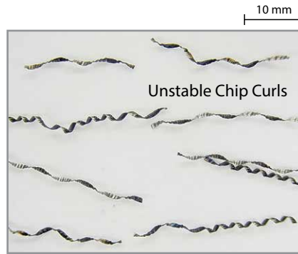
Competitor A (With Chipbreaker)
