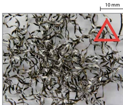
Without Chipbreaker (Conventional)
