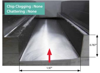
Cutting Conditions : Vc = 130 sfm, D.O.C. × ae = 0.787" × 1.97" (Slotting), fz = 0.003 ipt ø50mm (5 Flutes), Wet (External and internal coolant) Workpiece : Ti-6Al-4V Machine : BT50
