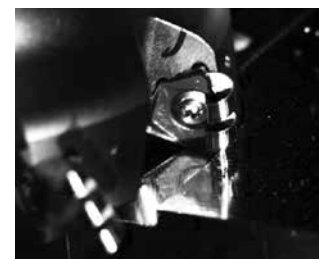
Properly Curled Chips (The Photo was Taken by a High Speed Camera)
