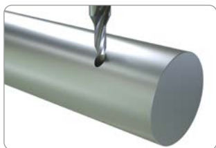
Eccentric holes on convex surfaces.
