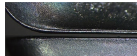
Cutting Length 91.9 feet Can Continue Machining Up to 150.9 feet
