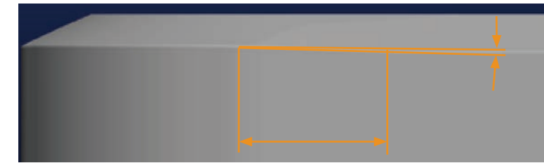
The Optimum Wiper Width Applying slight slope on the wiper cutting edge reduces cutting resistance.
