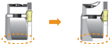
Analysis by Simulation Deflection Measurement : .0017 inch (0.044 mm) Analysis by Simulation Deflection Measurement : .0005 inch (0.013 mm)
