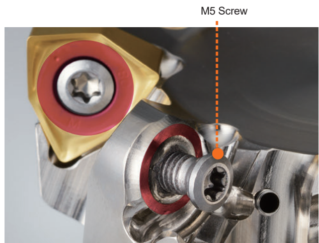
Conical shaped seat and M5 screw.
