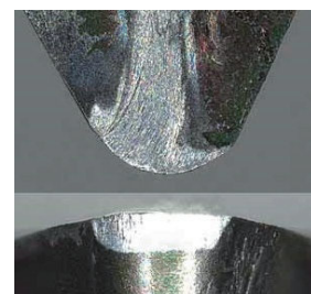
Conventional DLC Wear progresses due to peeling
