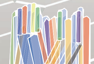
Conventional CVD inserts Grain size and growth direction are uneven.
