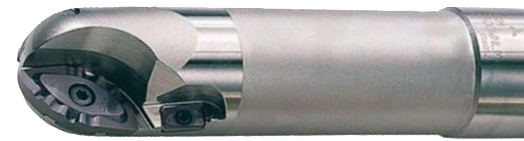
SRM2 Ø50 Ball nose, indexable insert end mill for heavy roughing.
