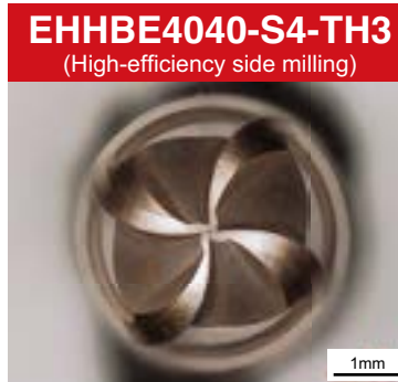
Flank wear : 0.015mm
