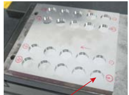
Machining shape \phi .347 inch \times Depth .059 inch
