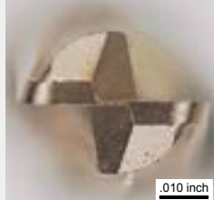
Flank wear : .0002 inch (0.005mm)
