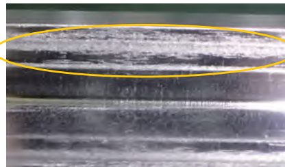
Biting of Chips Occurs Conventional A
