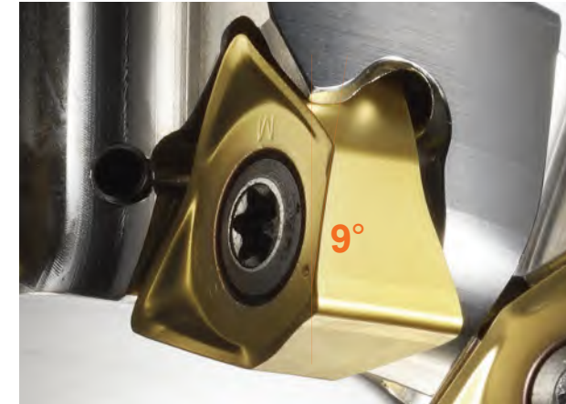
Axial Rake Angle of 9°
