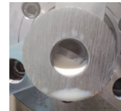
Steel shank without coolant thru + SLV sleeve
