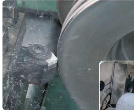
【Gray cast iron, Finishing, Dry cutting, White ceramic】
