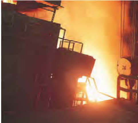
Electric arc furnace
