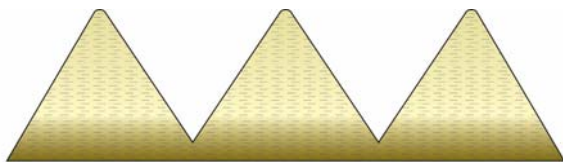
Figure 2: Grain structure of cut thread
