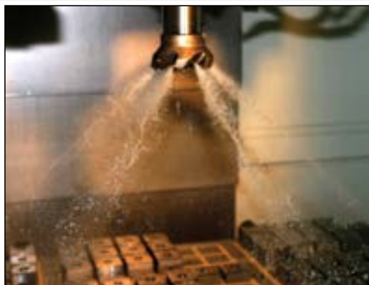
CoolBLAST arbor screw provides coolant path.
